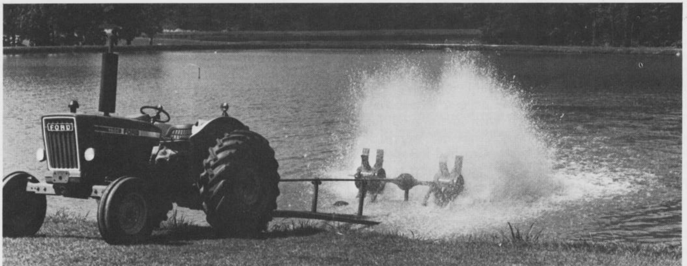
FIGURE 6. A PADDLEWHEEL AERATOR.
