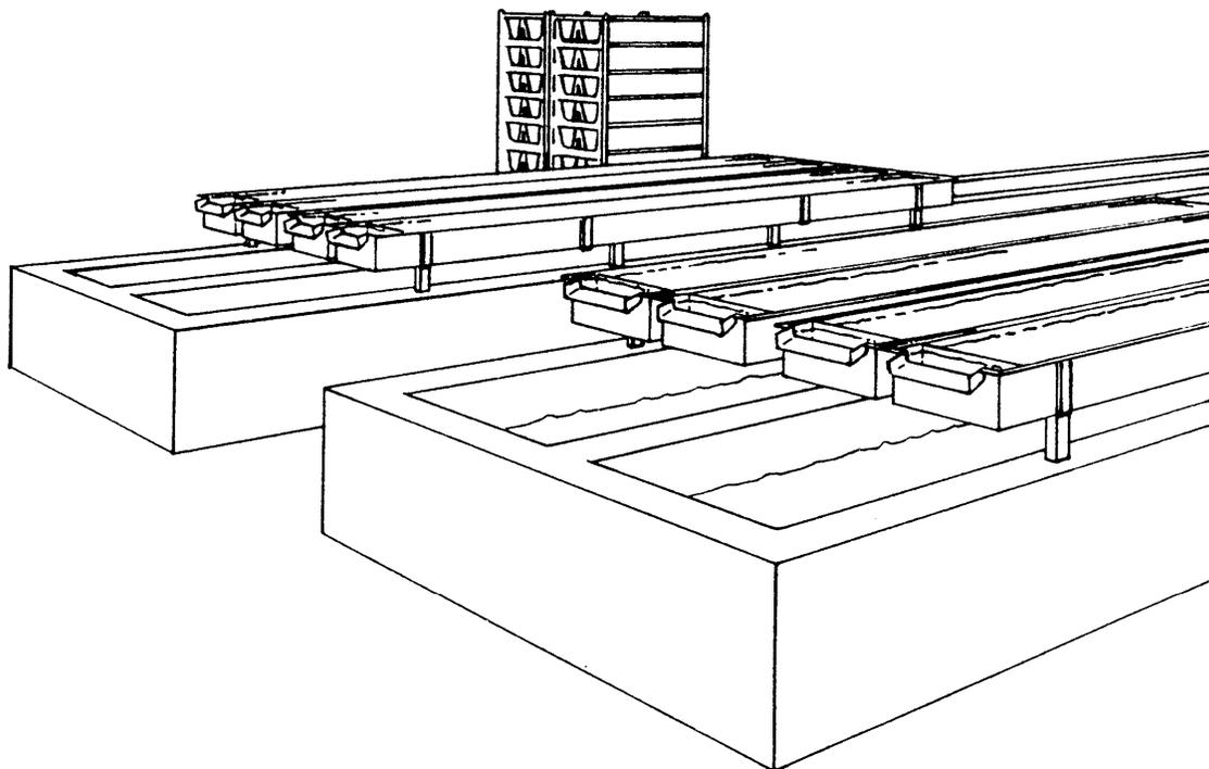
*Figure 2. Typical small trout hatchery, with hatching trays, fry troughs and fingerling tanks*
